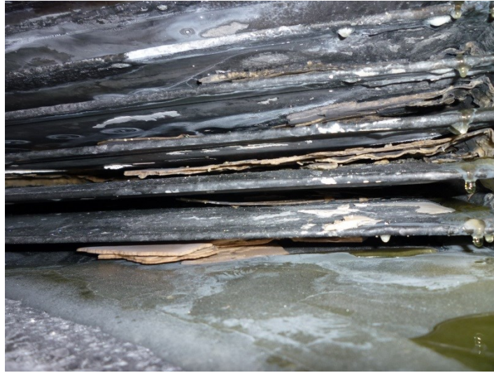
Figure 1. Scale on the heat transfer wall.
